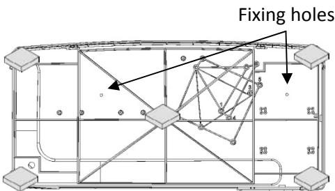
**i** The anti-vibration blocs are fitted under the base of the heat pump.
