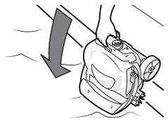
While holding Spabot under water, wave the cleaner to release any trapped air bubbles. When the bubbles stop, release the cleaner. The cleaner will sense it is in water and begin to move.
