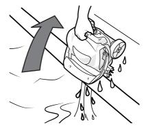
3. Set the cleaner on its back to accelerate water drainage.
