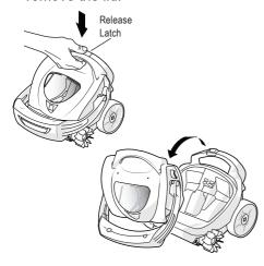
Press the filter cover release to remove the filter canister.
