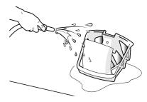
NOTE: Fine debris can impact the canister filtration and cleaner performance over time. Periodically, clean thoroughly with soapy water and a soft bristle brush.
