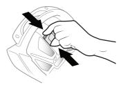
3. Empty debris and rinse the filter canister with fresh water. Reattach canister to the lid.
