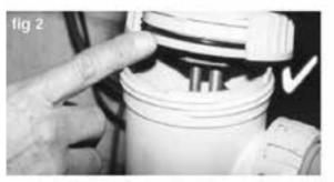
The 'O' ring must be fitted to the control head against the retaining edge before fitting to heater body. Do not rely on locking ring to pull head and body together. Use downward pressure while tightening locking ring, making sure that locators engage correctly. Hand tighten only.
