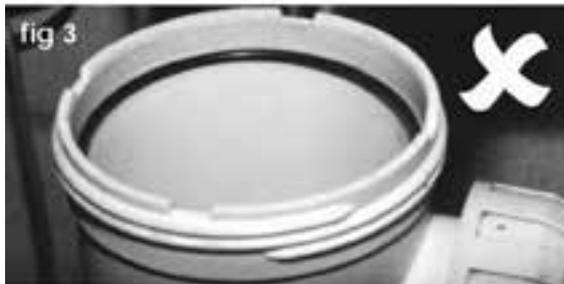
DO NOT assemble heater with 'O' ring as shown. This will dislodge when head and body are engaged causing water damage to the electronics. However, lightly lubricating the inside of this lip is permissible & will help assembly.
